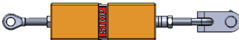
Figure B 1a - Shock absorber with a released fall indicator
